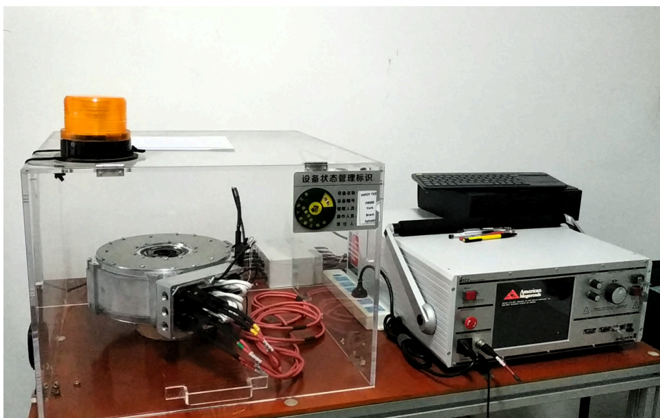
Figure 2.21: High-voltage test (M-OP110)
